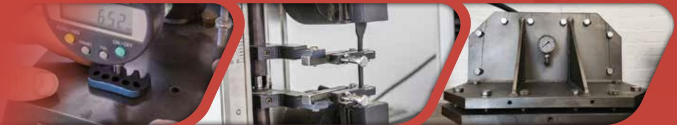
Gaskets are also tested at our UK headquarters in specially designed test rigs, which replicate the build of a segment ring in order to measure their performance.
