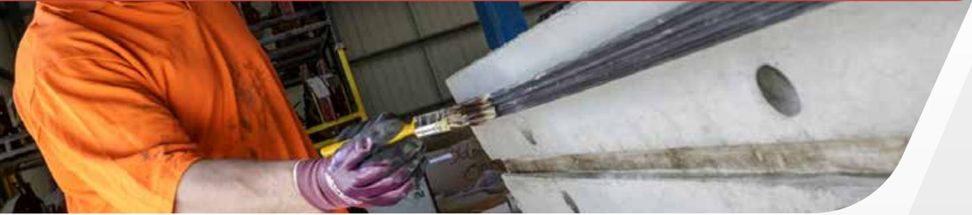
Traditionally the industry has used elastomeric gaskets that are glued into grooves cast into concrete segments which have a groove in place to accommodate the gasket. VIP manufacture a range of profiles which are compatible with many pre-existing segment moulds.
