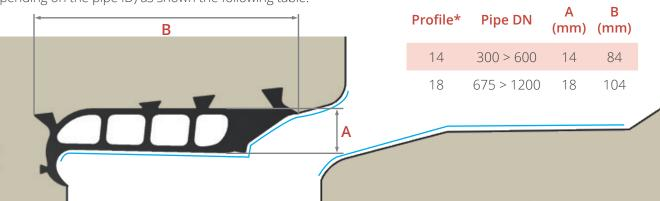
To reduce friction and ensure an easy connection of the pipes on site, it is important to clean and lubricate both the seal and the spigot section of the pipe (highlighted in blue on the image above). A minimum force of 2.5 times the pipe weight is required (under normal conditions) to connect each section.
