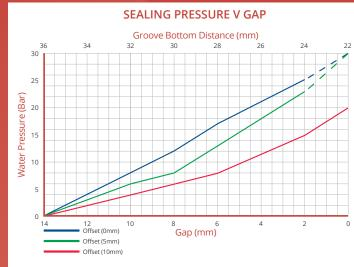
Diagram showing typical pressure curve
