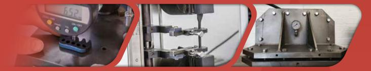
Gaskets are also tested at our UK headquarters in specially designed test rigs, which replicate the build of a segment ring in order to measure their performance.
