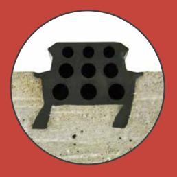
Cast-in seals 'anchor' themselves to the segment as the concrete surrounds the legs at the base of the seal. This process ensures a consistent positioning of the gasket around the segment.
