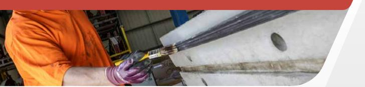
Traditionally the industry has used elastomeric gaskets that are glued into grooves cast into concrete segments which have a groove in place to accommodate the gasket. VIP manufacture a range of profiles which are compatible with many pre-existing segment moulds.
