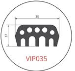
As per VIP's Cast-in gaskets, the Glued-in profiles have corner joints that can be manufactured to match the angles of the segment design. The corners are formed using an injection process using moulds that match the exact profile of the extruded gasket, ensuring that when the segments are joined together, the gasket can collapse into the groove and the load on the corners is equal to the rest of the gasket.
