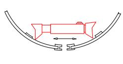
The pressing force that is required for the installation of internal seals depends on the following:
